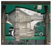
**Self-propelled hydrostatic drive** with intuitive forward & reverse drive controls eliminate pushing to reduce fatigue. Simple auto release switch for transport in off position.
