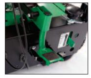
**Foot pedal** for operator ease of use and improved blade depth and wear. Standard on OS901. Retro Kit available for older OS900 Series. (Part No. 351611)
