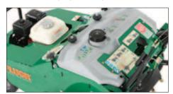
Water weight tank (PL2501 series) positioned directly over tines for better aeration depth and wheel traction in drier conditions. Full tank capacity is 40 pounds.
