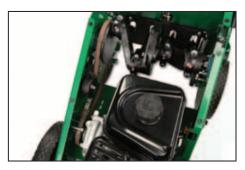
**Longer belt span** improves belt de-clutching and increases belt life. (PL1802V)
